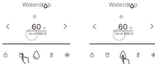
**Step 4:** Tap the temperature key "水温" to select the desired water temperature: cold water (41-50°C), ambient water (real-time temp), 45°C, 60°C, 85°C or 95°C.
