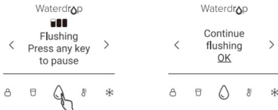
**NOTE:** The icon "■■■" indicates ongoing flushing, while "□□□" indicates completion.
