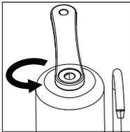
Place the system in the water sink, and use the wrench to unscrew the filter housing from the top (there will be water between the filter housing and the base).
