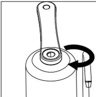
Screw the filter housing into the base by hand and tighten it with the wrench.
