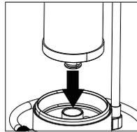
Remove the expired filter from the system and insert the new filter into the base. Make sure the sealing ring has been installed firmly, and the plastic film of the new filter has been removed.
